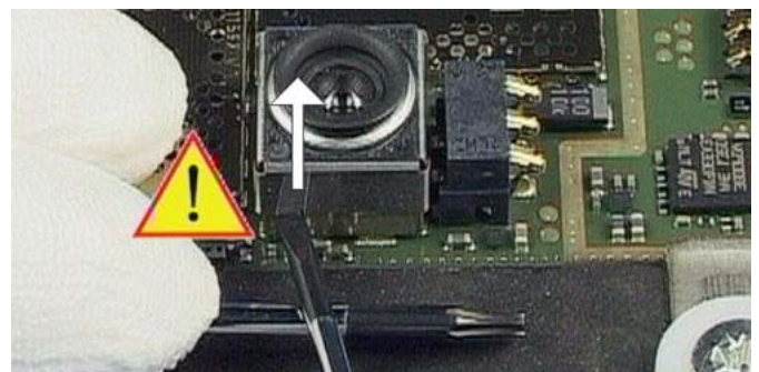
Use a slotted screwdriver as a lever to open the Camera Shield.
