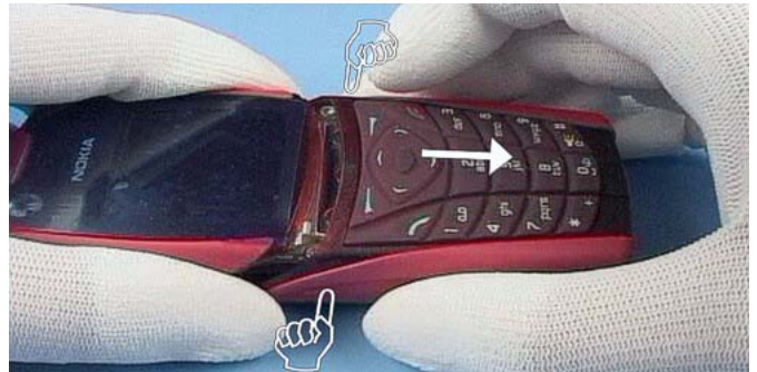
Press the grip markings on both sides of the B-Shell and remove B-Shell.
