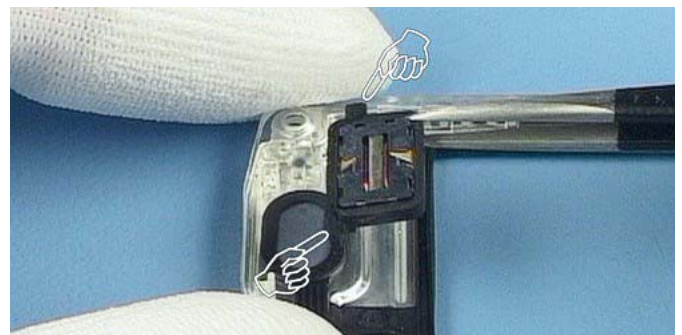
Remove the Speaker with Kirk Boot. Note the guiding when assembling.
